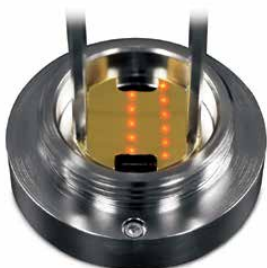
Laser reflections shown on the bottom mirror of the variable-path gas cell for pathlength determination.
