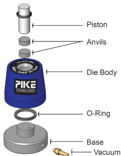
Evacuatable pellet press assembly.
