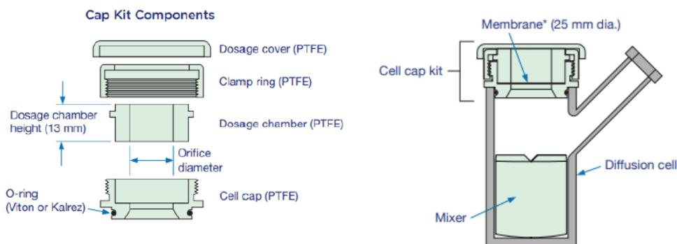
A diagram of the Phoenix vertical diffusion cell and cell cap (donor and dosage chambers)
