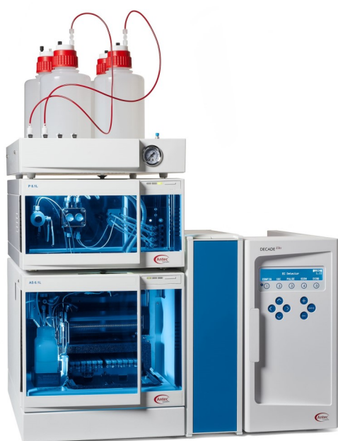
Figure 8. Recommended instrument configuration for this application: the ALEXYS Carbohydrate Analyzer. The system consists of a P6.1L quaternary LPG pump capable of running gradient program, an AS6.1L autosampler, a CT2.1 column thermostat, an ET210 Eluent tray for nitrogen blanketing, and a DECADE Elite electrochemical detector. The ALEXYS Carbohydrate Analyzer can be fully controlled by different Chromatography Data System (CDS) software, namely DataApex™ Clarity™ CDS (version 8.3 and up) or Thermo Scientific™ Chromeleon™ CDS (version 7.2 SR5 and up).
