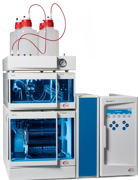
Figure 4. Recommended instrument configuration for this application: the ALEXYS Carbohydrate Analyzer. The system consists of a P6.1L quaternary LPG pump capable of running gradient program, an AS6.1L autosampler, a CT2.1 column thermostat, an ET210 Eluent tray for nitrogen blanketing, and a DECADE Elite electrochemical detector. The ALEXYS Carbohydrate Analyzer can be fully controlled by different Chromatography Data System (CDS) software, namely DataApex™ Clarity™ CDS (version 8.3 and up) or Thermo Scientific™ Chromeleon™ CDS (version 7.2 SR5 and up).
