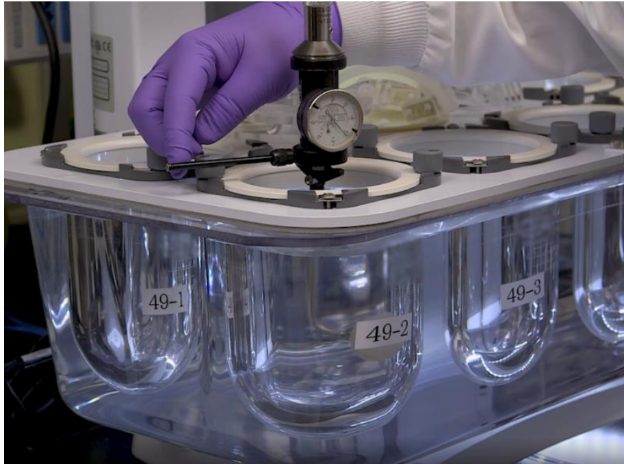
Figure 5. Using a centering gauge to determine the deviation of the vessel central axis from that of the stirring element at approximately the 500mL fill level.
