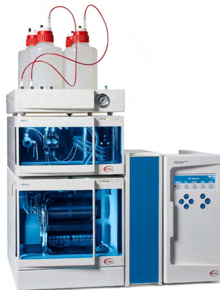
Figure 1: ALEXYS Carbohydrates analyzer consisting of the ET 210 eluent tray, P6.1L analytical pump, AS6.1L autosampler, CT2.1 column thermostat and DECADE Elite electrochemical detector.
