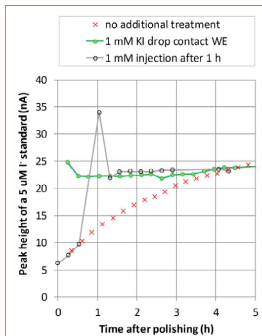
**Figure 11:** Response of iodide at a FlexCell equipped with a silver working electrode after different treatments. Background current was set to about 25 nA ( $E_{\text{cell}}$  -100 mV). Separation conditions as in Table 1.
