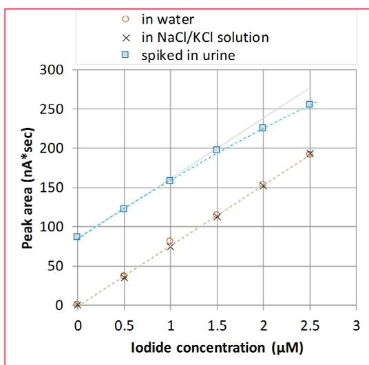
**Figure 8:** Response plot for iodide in water, in 150 mM NaCl/100 mM KCl, and spiked in urine up to 2.5 µM (317 µg/L). The dotted lines represent the regression lines with equations given in Table 4. The light grey line has the same slope as the non-urine data to help see the curvature. Data based on analyses with conditions as given in Table 1.
