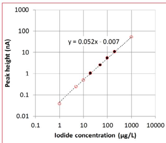
**Figure 7:** Log-log response plot for iodide peak height, spanning 3 orders of magnitude. The dotted line represents the linear regression line. The filled circles represent concentrations indicating nutritional deficiency boundary levels as given in reference [1]. Data based on analyses with conditions as given in Table 1.
