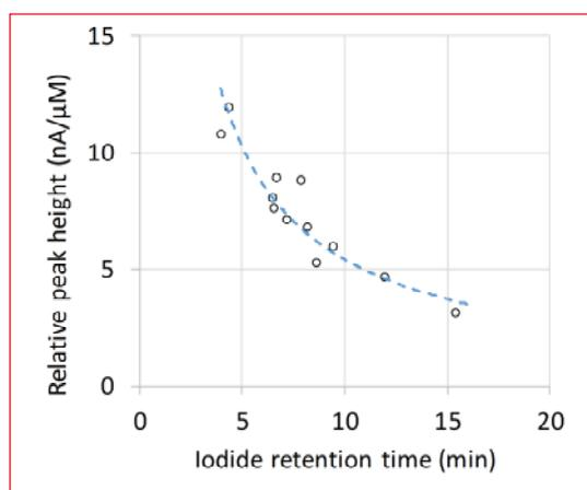
**Figure 4.** Inverse relationship between peak height and retention time (with peak area about the same for each data point).
