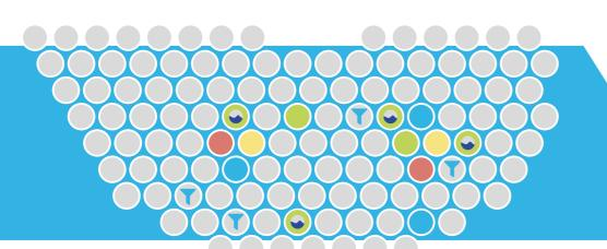
Rack for positioning accroTubes and filters. The tubes can be loaded with samples, solvents, or powders (as reagents)
