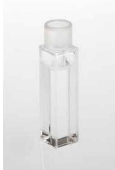
10 mm far UV quartz fluorometer cuvette with polished faces at 90° containing ultra-high purity water, permanently sealed by heat fusion.
