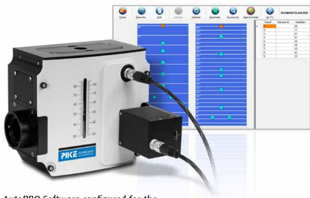
AutoPRO Software configured for the VeeMAX III with automated polarizer.
