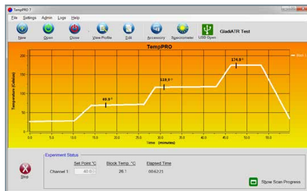
If PC control is desired, PIKE TempPRO™ software can be used for graphical setup and automated data collection with most FTIR spectrometers for thermal experiments.
