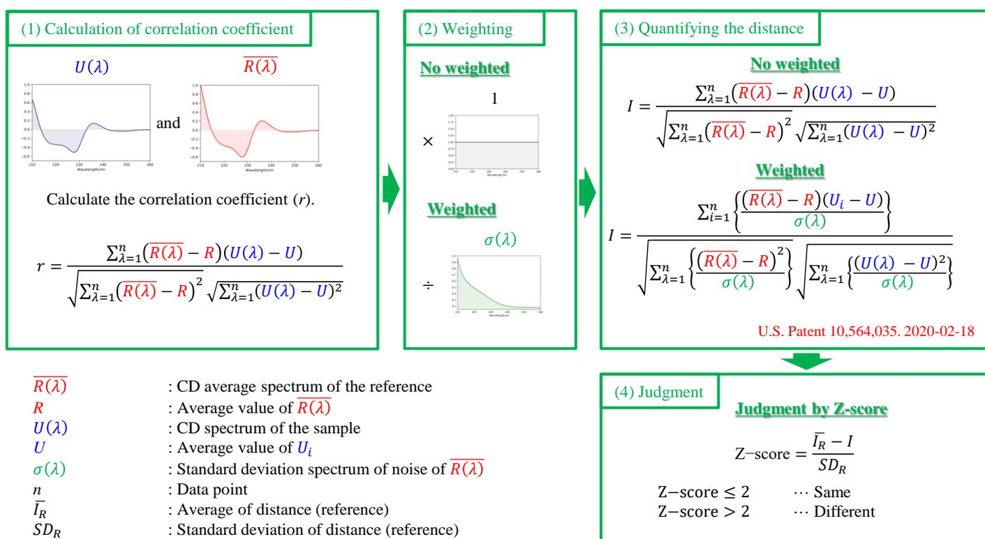
Figure 1. Analysis steps for determining the spectral differences between the reference and the sample spectra.
