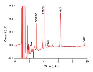
UHPLC-ECD chromatogram of rat prefrontal Cortex  $\mu$ -dialysate (after administration NA re-uptake inhibitor).
