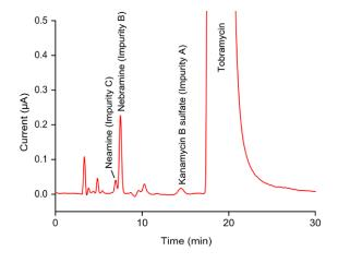
HPLC-ECD chromatogram of Tobramycin antibiotic, composition and impurity analysis according EP monograph. Column: 4.6 mm x 25 cm SDB copolymer. Injection vol.: 20  $\mu$ L. DECADE Elite equipped with SenCell with Au working electrode and Ag/AgCl reference. Potential: PAD 3 step waveform. ADF 0.5 Hz. Other conditions see Application note 217\_032
