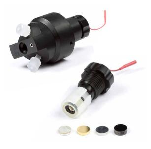
(MD), which can be quickly and easily exchanged. Magic Diamond (MD) also known as Boron Doped Diamond (BDD) is the workhorse and electrode of choice for oxidation reactions up to a maximum applicable voltage of 4.0 V. Pt and Au are typically employed for specific reactions such as hydroxylation or N-oxidation.
