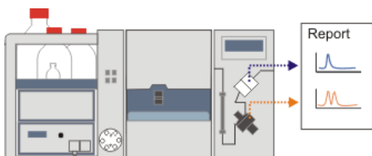
Fig. 2. Configuration for analysis of microdialysates using a DECADE II DCC with two cells in series. An oxidative reactor cell followed by a reductive VT03 cell (ox-red configuration).
