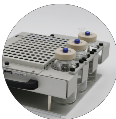
SRA-842 | Rack for sample vials Holds up to 120 sample vials and three flushing solvents (approx. 170 mL).
