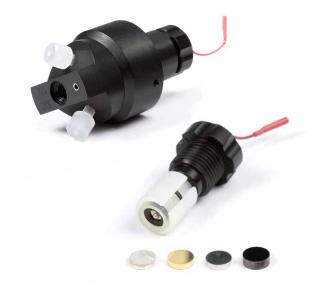
Au, Glassy Carbon (GC), and Magic Diamond (MD), which can be quickly and easily exchanged. GC is the workhorse and electrode of choice for oxidation reactions up to 2.0 V. For voltages > 2.0 V, MD a conductive diamond electrode is recommended as it can be used up to 4.0 V. Pt and Au are typically employed for specific reactions such as hydroxylation or N-oxidation.
