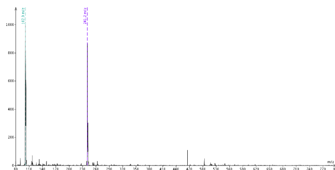
Figure 6. Mass spectrum of fractions 4-7 (product) 77.4 mg, 0.32 mmol, 64%.
