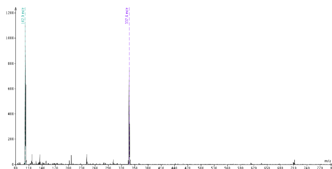
Figure 4. Mass spectrum of fractions 1+2 (dialkylated by-product) 31.3 mg, 0.09 mmol, 18 %.
