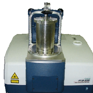
Fig. 1 Full vacuumed FT/IR-6300FV with LPC-12M-FV gas cell
