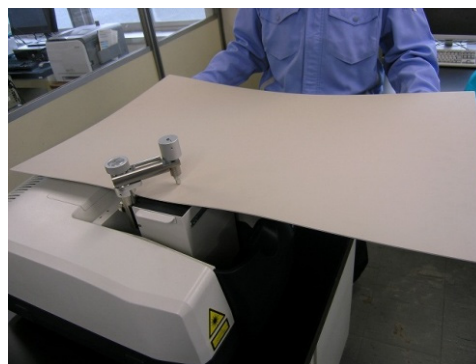
Fig. 3. A1 size sheet on ATR PRO510T-S
