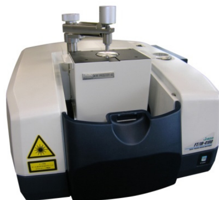
Fig. 2. Single reflection ATR for large-sized sample (FT/IR-4100 with ATR PRO510T-S)
