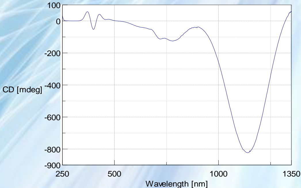
Fig. 1: CD spectra of mix solution including Nickel Sulfate and Rochelle Salt Cell path :10 mm Instrument range: 250-900 nm (J-1500) 900-1350 nm (J-730)
