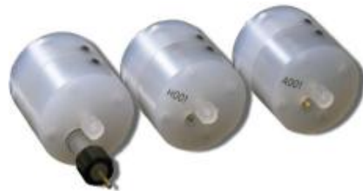
Fig. 1. Flow cell with salt bridge, HyREF and ISAAC REF (from left to right).
