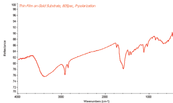
FTIR spectrum of an ultra-thin film on a reflective substrate using p-polarized IR beam.
