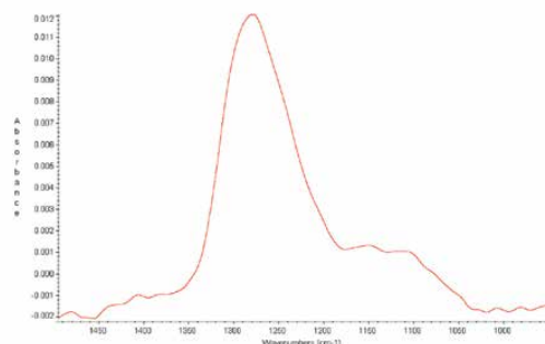
FTIR spectrum of an 18-angstrom thick lubricant on a hard disk measured in 15 seconds using an MCT detector.
