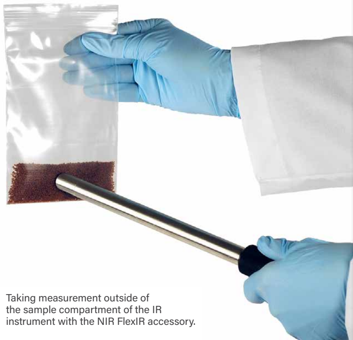
Spectra of incoming pharmaceutical materials measured and verified with the NIR FlexIR accessory.
