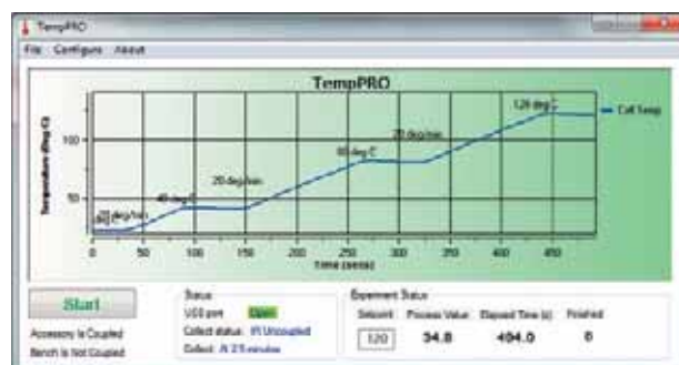
Selection of the digital control module, PC control includes PIKE TempPRO™ software for graphical setup and automated data collection for thermal experiments.
