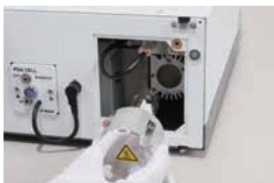
Front panel access for easy lamp replacement
