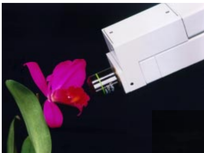
RMP-100 Raman Micro-Probe allows high-resolution Raman spectra to be obtained at locations remote from the spectrometer
