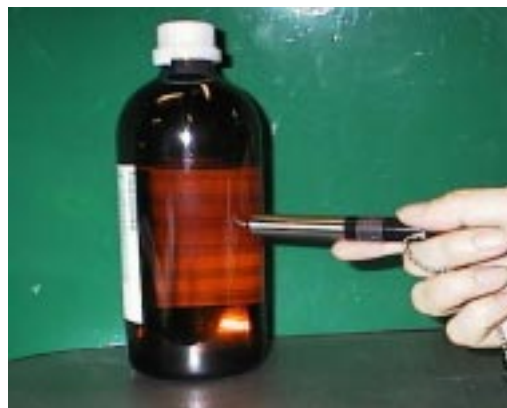
Using a Raman probe to examine a bottle's contents
